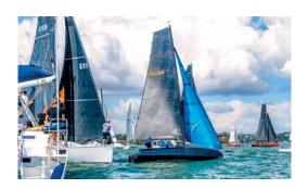
"When we designed it originally, it had a chine running the full length but rising slightly in profile at the aft end where it would flatten out once heeled," Houghton says. "We then decided to drop the chine further in profile, to flatten the aft sections. The chine came out exactly where the waterline should be, so that was perfect."
