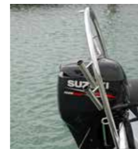
The stainless roll bar acts as towing point for water toys and rod holder mount.
