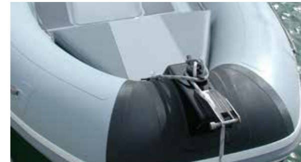
The anchor tackle comes over the tubes in a large stainless roller.
