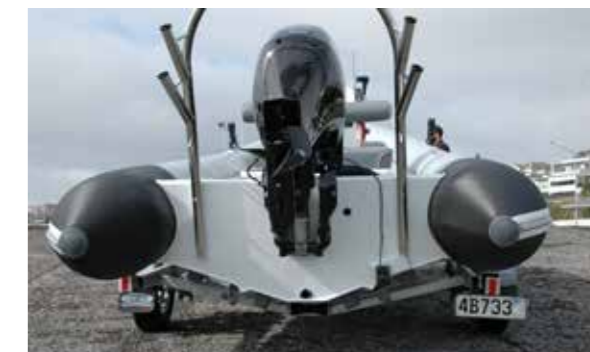
The 550 is based on a deep vee 22 deg alloy hull with pressed strakes.
